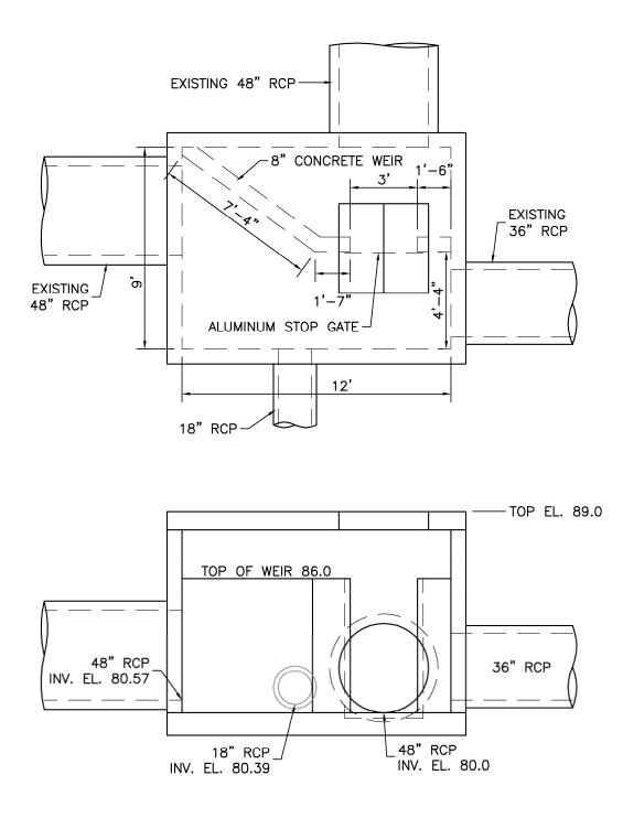
Figure 1-4. Schematic Details of the Diversion Structure.
