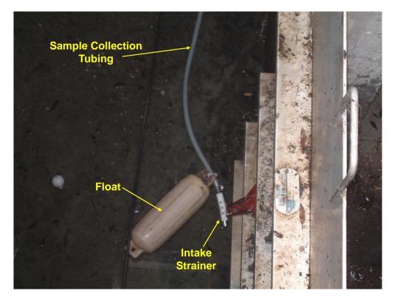
Figure 2-8. Modified Intake Strainer Attachment.
